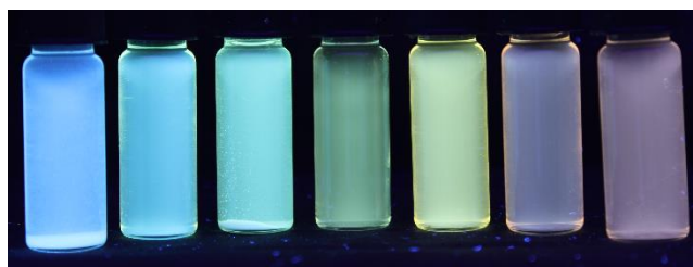
Figure 3-1. Positive emission solvatochromism of 4-(5-(4-(dimethylamino)phenyl)-1-methyl-1 H -pyrazol-3-yl)benzonitrile ( 10q ).
